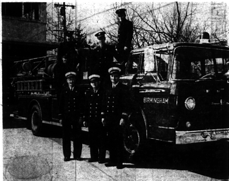
BIRMINGHAM'S FIRE department has come a long way from the first hand-drawn carts used back in 1910. The department's newest engine, Ladder #34, is pictured above with some of the members of the present 37-man crew. The engine, an American LaFrance Quint with a 750 GPM pump and a 75-foot aerial ladder, was purchased in 1961.
