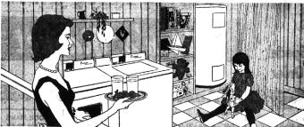
closet. Because there's no flame, an electric water heater doesn't need air flow to support combustion, or a vent to carry off fumes. There's even a table-top model you
