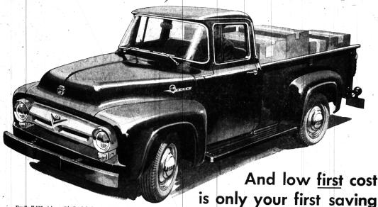
Ford's F-100 pickup with the 8-ft. box is the biggest in the half-ton field-up to 19 cu. ft. more loadspace than the others. Regular 6½-ft. box with a full 45 cu. ft. capacity also available.
