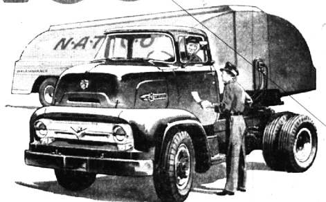
Ford C-900 with 212-h.p. V-8 has 4-barrel carburetor and dual exhausts to give you power when you need it.
