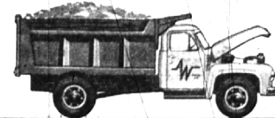
NOW 1 TON MORE GVW —Sales leader in its weight class, Ford F-800 now has GVW increased to 24,000 lbs. with heavy-duty rear springs, 170-h.p. Short Stroke V-8. Power Steering optional; low extra cost.
