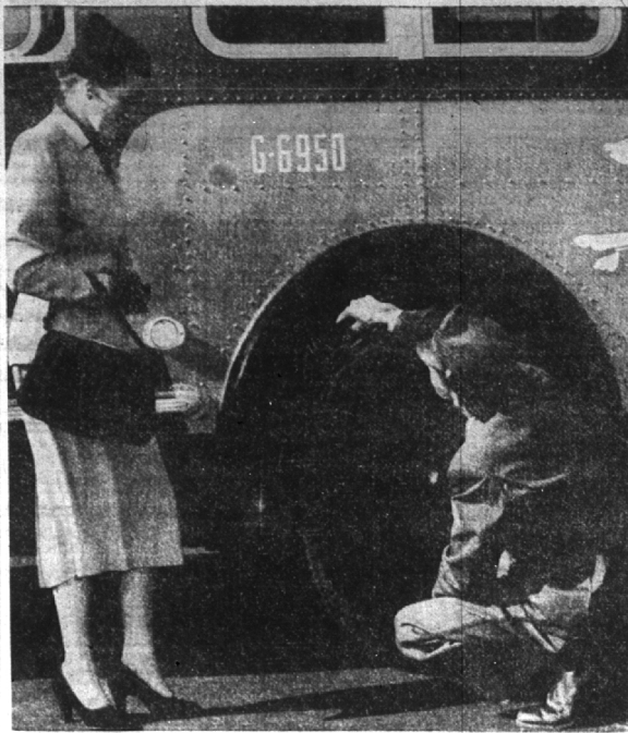
GREYHOUND DRIVER Charles Szyperski shows passenger the location of an air-ride suspension unit on one of the new Greyhound suburban buses recently placed in service in Birmingham and several other Detroit area communities. According to R. W. Budd of Vaughan road, Bloomfield Hills, president of Great Lakes Greyhound Lines, air suspension ride presents a totally new concept in motorbus engineering. The coach has no metal springs. Passengers literally ride on air. The coach body is supported by eight giant air cells which breathe through metering devices. Road shocks are absorbed with squeakless, effortless compensating action. And special leveling valves act to produce the same comfortable ride in every seat.
