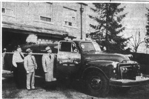
BLOOMFIELD TOWNSHIP OFFICIALS proudly inspect their new fire truck which increases the township's fire equipment to three trucks. The 1,000-gallon tanker is equipped with a 300-gallon per minute high pressure pump and is mounted on a 2½-ton G.M.C. chassis. Taking their turns at the cab, from left to right, are Police Chief Clark Green, Supervisor David E. Anderson, Treasurer Arno L. Hulet and Fireman Lester Allen. (Eccentric Staff Photo)
