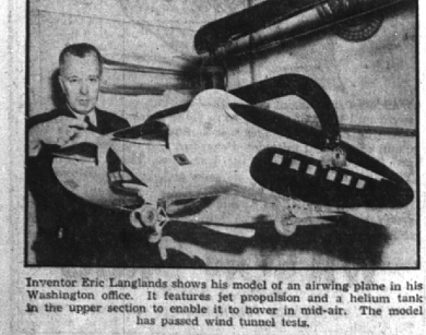
Inventor Eric Langlands shows his model of an airwing plane in his Washington office. It features jet propulsion and a helium tank in the upper section to enable it to hover in mid-air. The model has passed wind tunnel tests.
