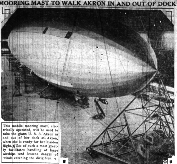
This mobile mooring mast, electrically operated, will be used to take the giant U. S. S. Akron in and out of her dock at Akron, when she is ready for her maiden flight. Use of such a mast greatly facilitates handling of large airships and lessens danger of winds catching the dirigibles.
