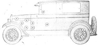
1 Advanced Six-Cylinder L-Head Engine 2 Harmonic Balancer 3 Oil Filter Air Cleaner 5 Full Pressure Oiling 6 Automatic Spark Control 7 Four-Wheel Brakes 8 Larger Balloon Tires 9 Duco Finish 10 Dimmer on Steering Wheel
